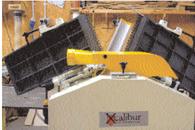
You can't start the machine with the tables up unless the hood is in place
